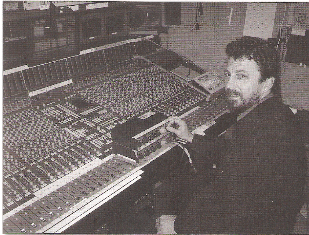
Figure 2.2 When this digital mixing desk went dead, Mark Butler rigged two small Shure mixers together to get the job done.
